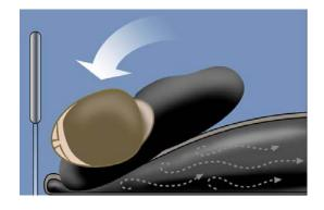
Standard *fully air-filled mattresses* collapse as the patient rolls toward the edge, directing the patient into siderails or onto the floor.
