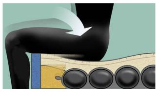
The **Safety Edge** is a two-part bolster system surrounding the air tubes on all PressureGuard products. When the user rolls toward or sits on the edge of the mattress, the inner of the two parts bends in toward the center of the mattress, while the outer part resists collapse.
